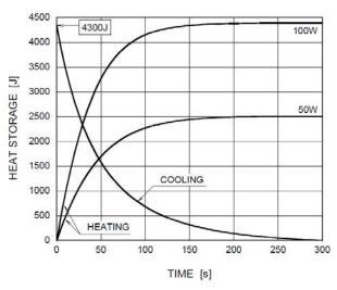
Heating/Cooling Curves of the Toshiba D-041 anode
