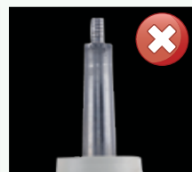
Worn screw thread with non genuine tips
