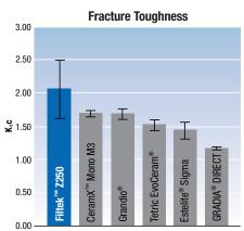
Results of a single notch fracture toughness test proves Filtek™ Z250 Universal Restorative is more fracture-resistant than leading composites tested.
