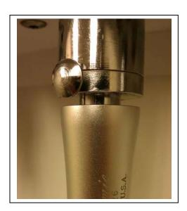
10. You may adjust the pressure in the reservoir to adjust the amount of air pressure that is supplied to the hand piece. Pull the knob outward to unlock it. Turn the knob counter clockwise to lower the pressure. Turn the knob clockwise to increase the pressure. Reference the air pressure gauge on the side of the unit to verify the set pressure.
