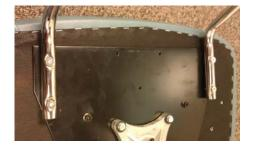
6. Turn the stool on its side and begin to install the armrests. Use the 6 bolts and washer sets to firmly fasten them in place.
