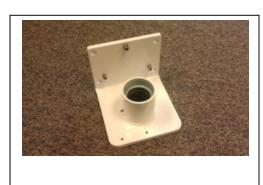
2. Mount the bracket in the desired location. A minimum requirement of 14" from the back side of the cabinet, to the inner edge of the bracket is required. This is to allow space for the delivery unit head to have ample space from the wall / cabinet backing.
