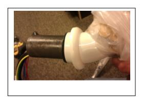
5. Guide the tubings through the mounting bracket. Then slide the flex arm into place.
