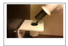
6. Once the arm is in place verify that the delivery unit arm is not drifting. If drifting is occurring make the proper adjustments to the leveling set screws on the mounting plate.
