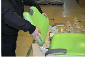
8. Install the seat cushion onto the seat frame. Make sure you align the mounting points before sliding into place.
