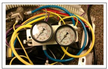
22. Once air and water pressure are set, you may now make adjustments to the syringe blocks if necessary. Also check your handpiece pressure and adjust accordingly.
