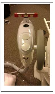
5. Verify the PMU is level before tightening the set screws on chair bracket. There are 8 set screws that will be used for leveling. If the PMU is not level the unit arms may drift. Small adjustments to the set screws will level the PMU. Level the PMU in the following directions. (left to right and front to back).
