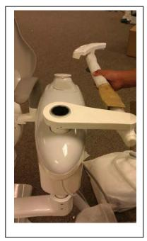
Turning this screw clockwise will raise the angle of the arm. Turning counter clockwise will lower the angle of the arm.
