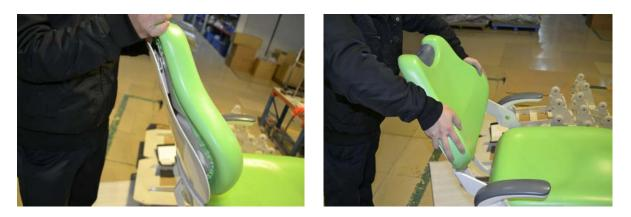
8. Install the seat cushion onto the seat frame. Make sure you align the mounting points before sliding into place.
