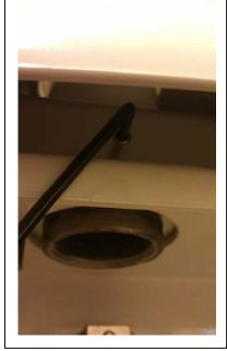
9. Take the delivery unit flex arm out, and place the additional cosmetic ring on it as shown below. Once in place, take all lines and feed it through the bushing assembly as shown. Verify that the arm seats completely down in the bushing assembly. Lower the cosmetic ring to cover the seam between the assistant's arm and the delivery unit flex arm.
