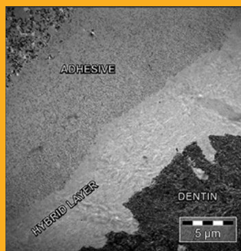
Figure 10: Dr. Bart Van Meerbeek. SEM of 3M™ Scotchbond™ Universal Adhesive to dentin in total-etch mode showing the adhesive film thickness to be in range of 5–10 microns.
