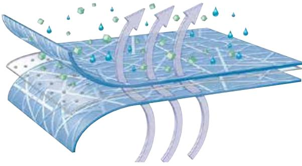
Outer layers - Spunbond polypropylene material that is cloth-like, yet tough and abrasion-resistant
