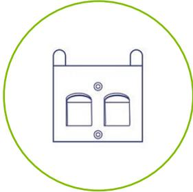
Secure STAY-DRY® Box to Bracket Using Tabs.
