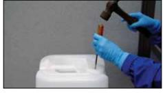
2. Use screwdriver and hammer to puncture the indentation at the center of the large cap. (Do not attempt to remove cap.)
