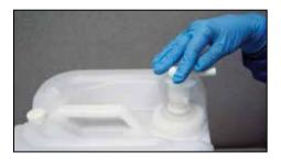
4. With the handle still facing the ceiling, screw the spigot tightly into the large cap.
