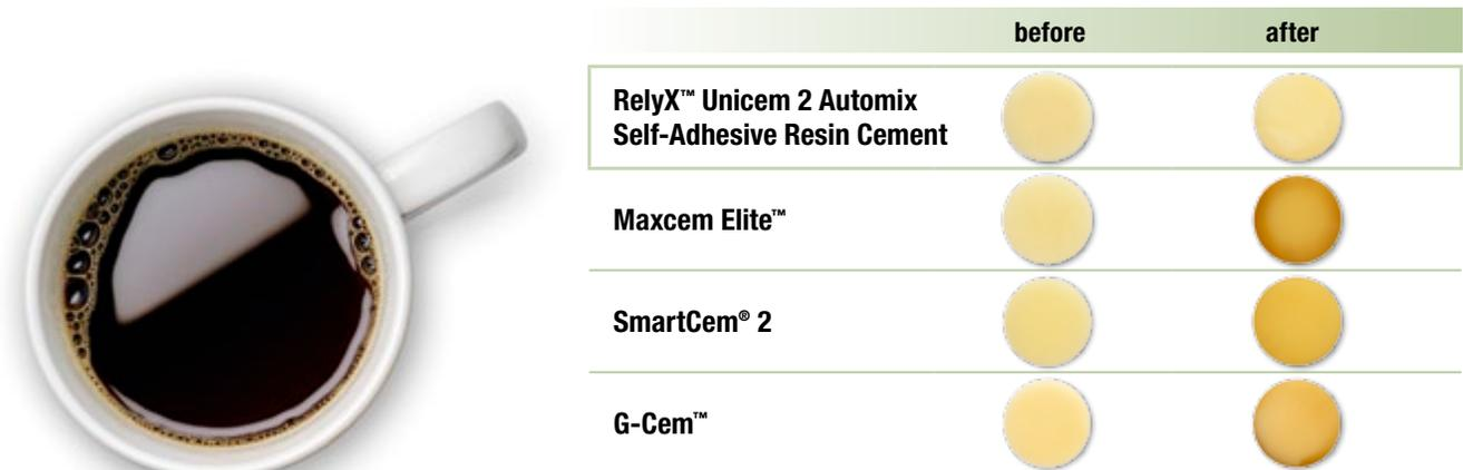
Fig. 19: Storage of cement specimen (light cured) in standardized coffee solution for 3 days. Source: 3M ESPE internal data
