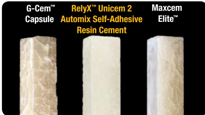
Fig. 18: Results of stress test on self-adhesive resin cements. All samples were self-cured and thermocycled 10,000 times. Source: 3M ESPE internal data
