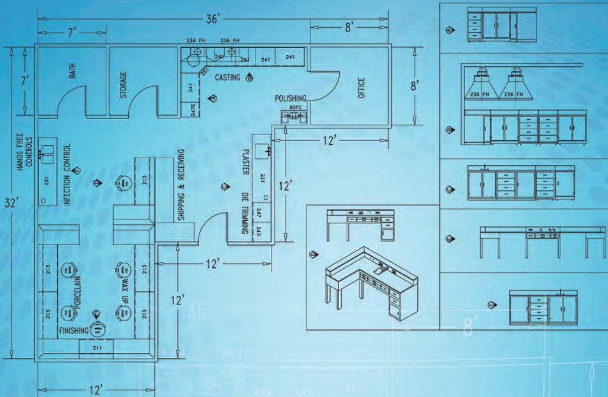
Handler's benches and cabinetry can withstand the rigors of the lab environment and are manufactured of 18 gauge steel with long-lasting Resistop® work surface.
