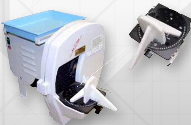
An Orthodontic Angulator Attachment for precise grinding of angles onto plaster or stone models. Easily set to desired angle up to 120 degrees from mid-line in 5 degree increments. Produces precise angled models for sturdy presentation. For Handler 10" [25cm] or 12" [30cm] Model Trimmer. **Orthodontic Angulator must be factory installed by Handler.**
