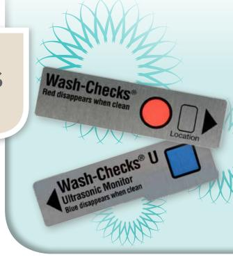
Colored test soil on strip is designed to parallel the removal of blood and bioburden from an instrument surface
