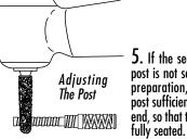
5. If the second tier of the post is not seated within the preparation, shorten the post sufficiently at the apical end, so that the second tier is
