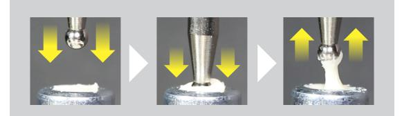
Figure 5: Test method: dipping of the plunger into the mixed paste and withdrawal immediately afterwards.
