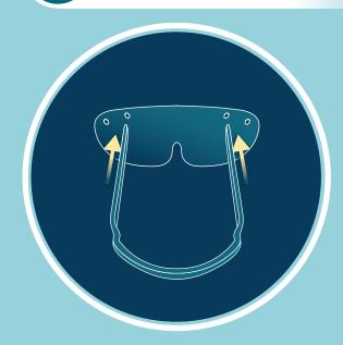
Slide frame (flat side down) through inside holes on lens
