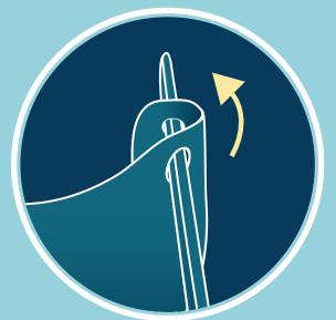
Slide lens forward into notches on frame
