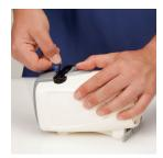
**Step 3:** Battery is properly seated when latching mechanism is slightly over battery edge. The battery fuel gauge (*LCD*) will be visible.
