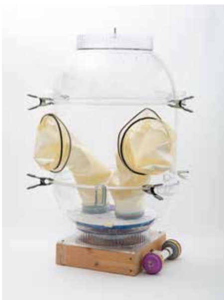
Figure 2 Sealed environmental test chamber for assessment of vapor containment.
