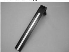
Fig. 2 -5: Beam adjustment jig
