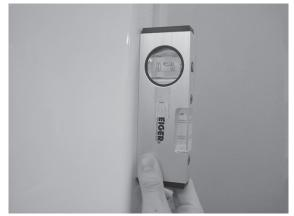
Fig. 3 -27: Checking for column lean
