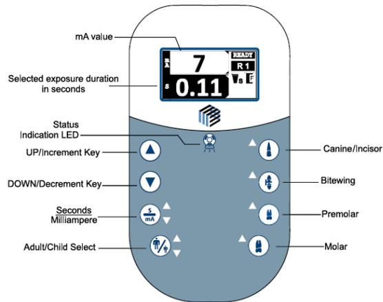
Figure 14. Intraskan DC Keypad Console with LCD Display
