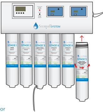
NOTE: After installing the new Stage 5 cartidge, please read the Monitor Reset Instructions to properly reset the Filter Monitor
