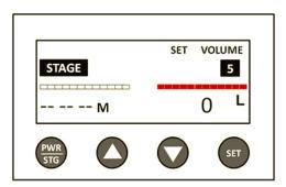
9. Use the Up Arrow key to adjust the liters to the value labeled on your Stage 5 Cartridge (1,000, 3,000, 7,000, or 10,000 L). The arrows can be held down to speed up the process.
