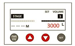
10. Hold SET until you hear two beeps. This will save the liter setting and will exit set mode. The display will show 0 L. THIS IS NORMAL. The liter clock starts from zero and will count upwards to the set value (3000 L in this example).
