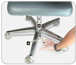
**3.** Turn over the seat/gas-cylinder assembly **4**. Hold open the latch **5** on the seat frame while lifting the gas-cylinder **6** out of the seat socket.
