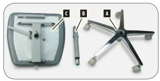
**4.** Hold open the latch **\( \Displayer)** on the seat frame while inserting the small end of the gas-cylinder **\( \Displayer)** into the socket. Make sure the latch fully engages with the lip **\( \Displayer)** on the end of the gas-cylinder.
