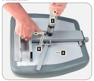
**4.** Turn over the base **A** and place it (wheels up) in the padded case with the latch **B** in any position EXCEPT the position shown with the "X" to prevent the latch from scratching the frame of the stool during transport.
