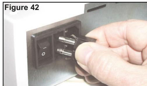
**NOTE:** The AEU-7000L/7000E features auto-sensing, global voltage compatibility. The fuse indicated is correct for 100V-240V 50/60 Hz line voltage.
